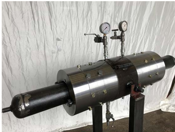
Figure 3: Hydrotest set up for smart hydraulic pipe to pipe connector
